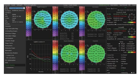
Scansys can decompose the complex corneal topography data of patients into quantitatively analyzable components such as Spherical Component, Decentration Component, Regular Astigmatism Component and Irregularity Component through Fourier Analysis, which can provide more scientific guidance basis for eye-care professionals to design refractive cataract surgery and personalized corneal refractive surgery plans.
